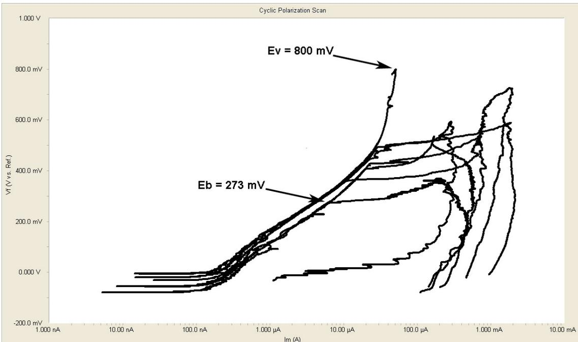
**FIGURE 5 - Seven (7) tests with highly variable results, with breakdown as low as 273 mV. One sample was completely passive, going all the way to Ev = 800 mV. Mean was 466 mV and standard deviation was 167. Note: tested conducted according to ASTM F 2129-06.**
