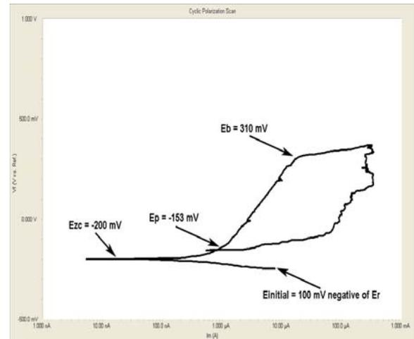
Testing in PBS. Breakdown at +310 mV.
