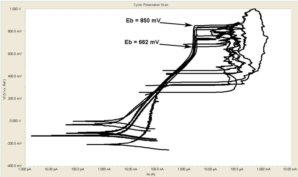
**FIGURE 4 - Seven (7) tests with good reproducibility. Eb ranged from 662 mV to 850 mV. Mean was 783 mV and standard deviation was 69. Note: tested conducted according to ASTM F 2129-04.**
