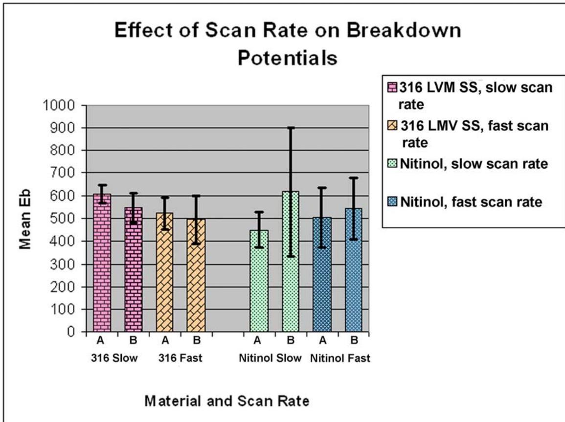
**FIGURE 3 - Mean breakdown potential for Type 316 stainless steel and nitinol tested at different scan rates. Note: testing was done at two different laboratories, denoted A and B. Data adapted from [10].**
